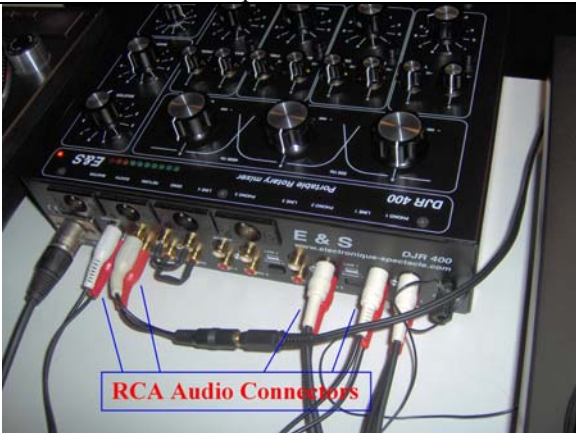
Audio Mixer Showing RCA Connectors [52]
