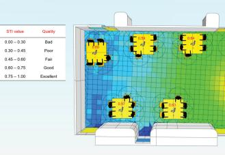
Figure 02: Acoustic simulation of speech sound level distribution and speech transmission index in a chort classroom at SUTD
