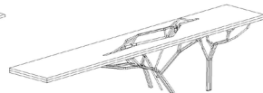
3 Creation of holes through the bench for the backrest, strengthening supports through increased bundling of rebars.
