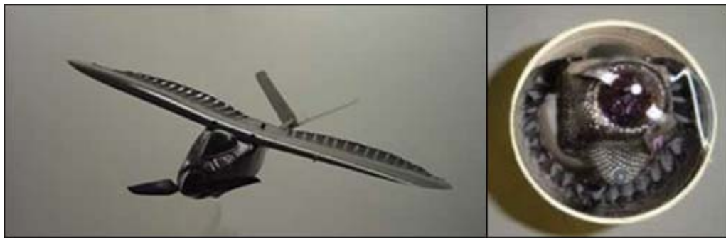
(a) (b) Figure 23. Tactical Mini UAV (TACMAV) (a) Deployed (b) Stored [26]
