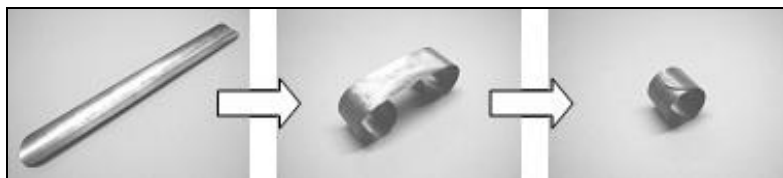
Figure 18. Metal insert from a “slap bracelet” [22]
