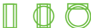
From left to right: The bottom, top and front views of a ring (the product)
