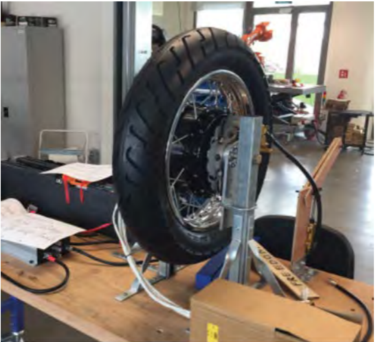
Prototype to test the performance of an electric drive train subsystem (motorized wheel).
